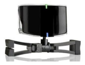
The camera is usually mounted on top of your monitor. The IR is reflected back to it from either one or three reflective dots (depending on which model of TIR you have) usually mounted on a ball cap. For extra fun make sure you leave your hat on with the Official Martian Fighter Pilot Antenna™ attached when you answer the door for the Pizza man.
