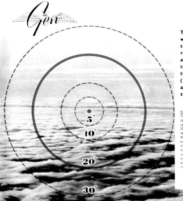
This diagram shows where the target ought to appear in the sight ring, according to the angle off. The nose of the target should touch the appropriate circle. (Notice that for 20 angle off, this circle is the sight ring).
